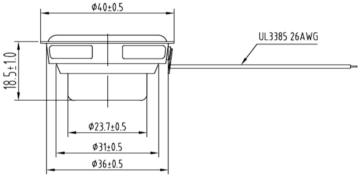
3,5 mm max for membrane moving at Max Power 3 mm max for membrane moving at Nominal Power
